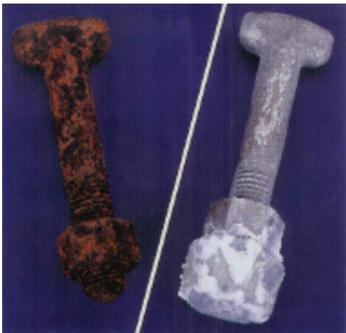
Submerged in concentrated salt water for 5,000 hours
